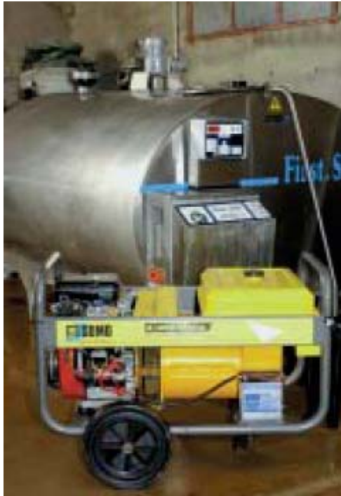
Figure 5. Portable Diesel Generator
