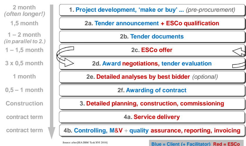
Figure 1: Outsourcing energy projects: Overview of workflow (client and ESCo) and typical lead times
