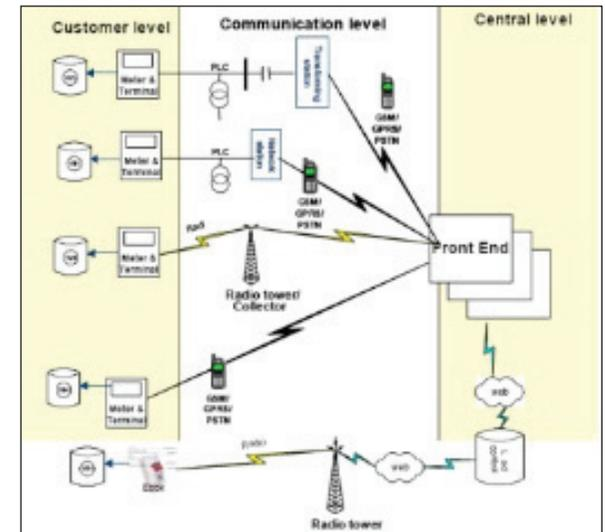
Figure 1. Information and Communication Technologies Used in the Pilot Project.
