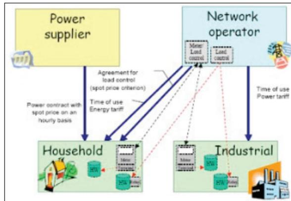
**Figure 5. Tariff and Load Control Arrangements for Skagerak Energi Nett AS**
