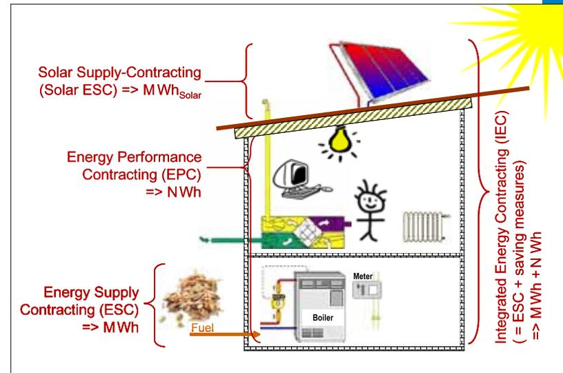
Figure 1. Scope of services of different ESCo models
