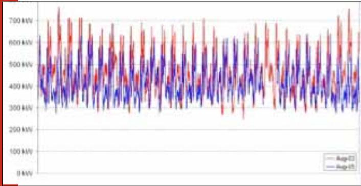
**Figure 4.** Load on the Crookwell to Grabine Feeder Before and After Implementation of the Bigga-Bigga Demand Management Project
