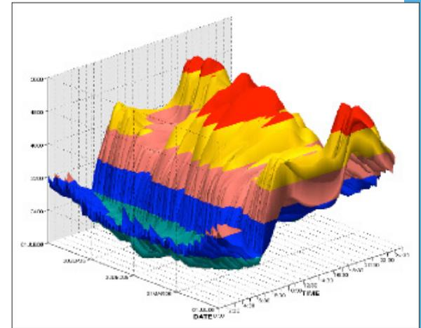
**Figure 1. Aggregated Load Profile for the EnergyAustralia Network, July 2005 to June 2006.**
