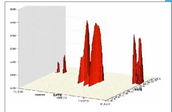
**Figure 2. Peak Loads above 5000MW on the EnergyAustralia Network, July 2005 to June 2006.**
