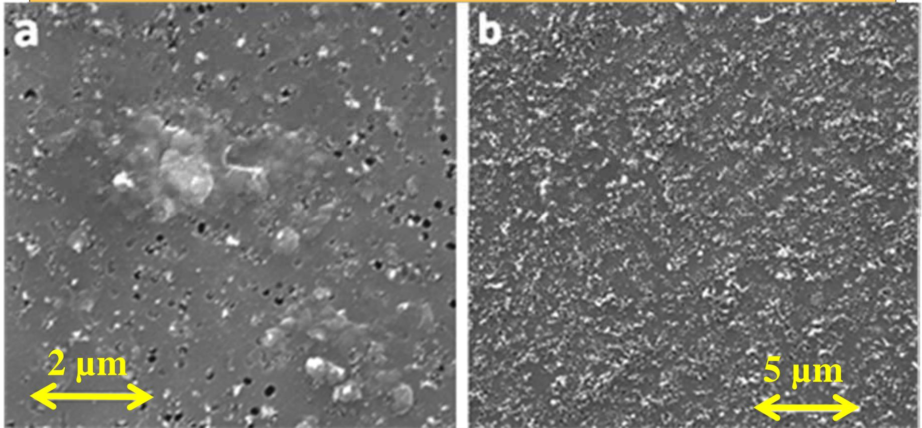
Presence of liquid condensed matter that has coalesced to form a layer which covers filter pores. Energy Dispersive Spectroscopy (EDS) showed that this thin film is dominated by C and O with traces of Mo, Zn and Fe.
