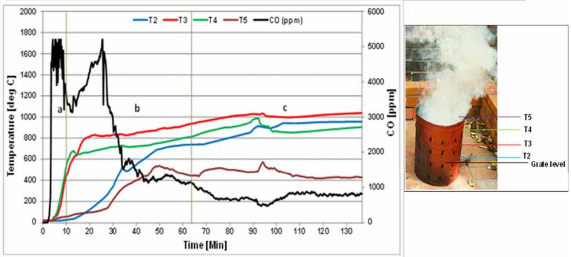
For the BLUD, ignition at the bottom creates an upward migrating pyrolytic zone that is starved of oxygen; generating a pyrolytic gas (CO, H<sub>2</sub>O, volatile and semi-volatile organic compounds), char and low flame temperatures (indicated by curve T5, Fig. 3, from 0 to 30 min after ignition).
