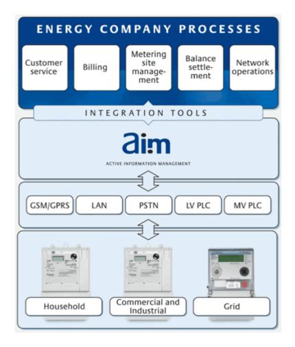
Enermet AIM not only does automatic meter reading but also refines the data for multiple purposes (e.g. billing). High quality AMR solution enables error-free and seamless data flow from meters to various IT systems (e.g. CIS).
