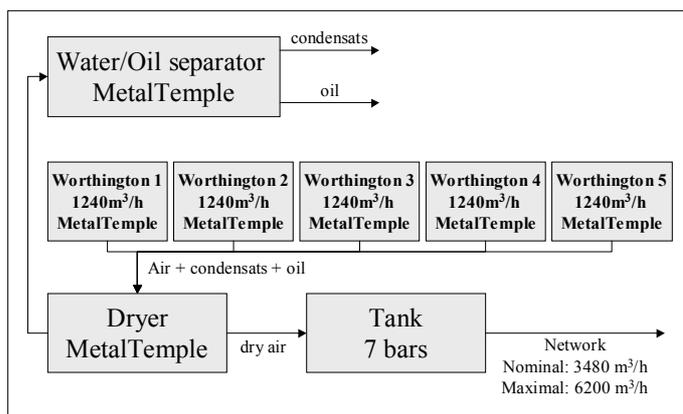
**Initially** – The compressed air station is composed of five Worthington compressors, one separator, one dryer and one tank.
