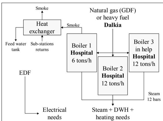
**Initially** – Three boilers worked for the heating of buildings, the production of DHW and its own needs of steam. The hospital purchased the totality of its electricity from Electricité De France.
