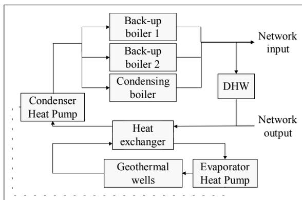
**After work** – geothermal is associated to a gas condensing boiler (heavy fuel as back-up) and the two old back-up boilers. A heat pump has also been installed to assist the geothermal energy. The installation produces the heat needed for the district heating and for the production of Domestic Hot Water.
