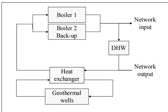
**Initially** – Geothermal is associated with two natural gas boilers (heavy fuel as back-up). The installation generates the heat needed for the district heating and for the production of Domestic Hot Water.
