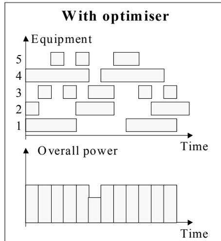
This device allows to manage power calls. Indeed, when the power called passes over the set point, the device switch the supply of certain equipments off. Also, when the power called passes below the set point, the device switch the supply of certain equipments on. The on/off priority depends on the process and the customer choices. Finally, load management with this device is possible only for equipments with inertia and is then favorable for thermal uses (furnace, cold group, ...).
