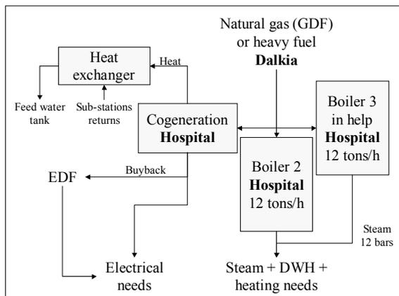
**After work** – Two steam boilers worked for the heating of the buildings, the production of DHW and its own needs of steam. Moreover, one cogeneration unit and a diesel fuel power generating unit are used for the production of electricity.
