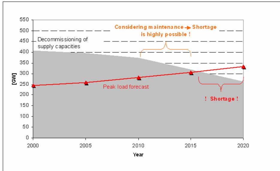
**Figure 1:** Decommissioning of capacities and peak load forecast for the central European Energy market.
