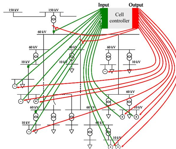
**Figure 10. Cell controller functionalities. Measuring and monitoring of load and production indicated by (green) arrows pointing towards the cell controller. Control actions on generators, load feeders and main power circuit breakers indicated by (red) arrows pointing away from the cell controller.**
