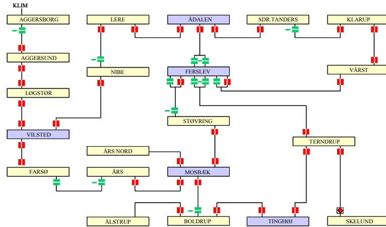
Figure 6. Typical 60 kV grid of a distribution company in western Denmark. Bluish (dark) substations are 150/60/10 kV substations. Yellow (light) substations are 60/10 kV substations. The radial operation is indicated by the position and color of the power circuit breaker symbols (red: closed, green: open).
