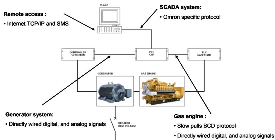
Figure 14. Typical control and communication system for a Gas Engine CHP unit.
