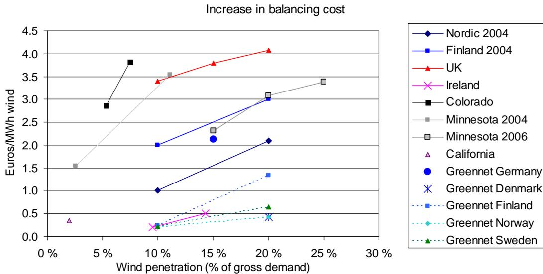
Fig 3. Results from estimates for the increase in balancing and operating costs due to wind power. The currency conversion used here is 1 €= 0.7 £ and 1 €= 1.3 US\$.
