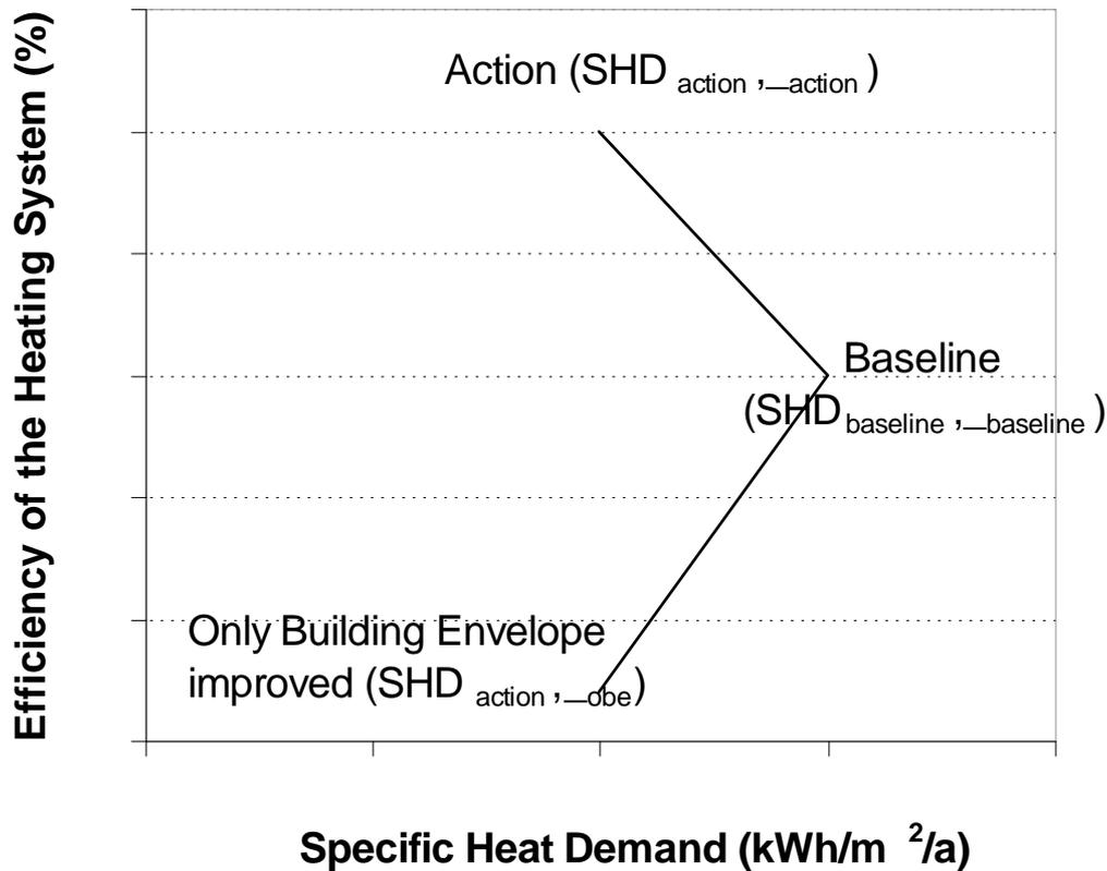
**Figure 4: Efficiency of the heating system vs. specific heat demand when the building envelope is improved and the heating system is replaced (case c) compared to the situation in which only the building envelope is improved (case b)**
