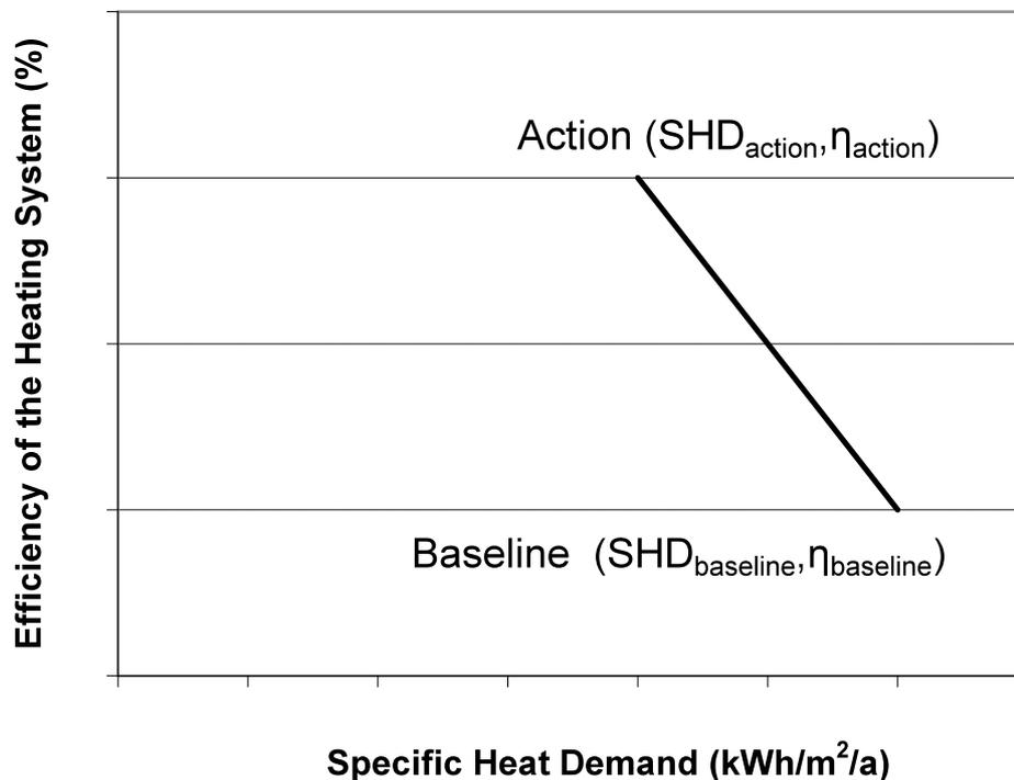
**Figure 3: Efficiency of the heating system vs. specific heat demand when the building envelope is improved and the heating system is replaced (case c)**
