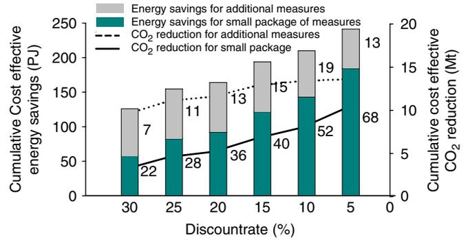
Fig. 5. Estimated primary energy savings and CO<sub>2</sub> emission reduction due to White Certificates for households in The Netherlands; cumulated results for the period 1995 to 2020 (each bar refers to the total period).
